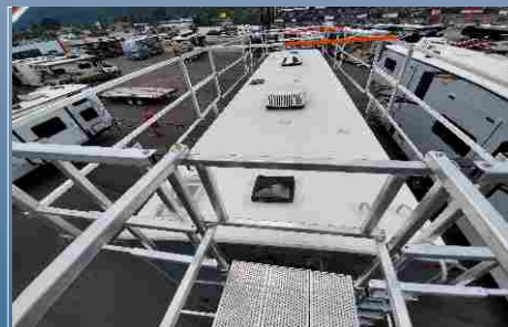
WRAP AROUND ROOFTOP CONTAINMENT
